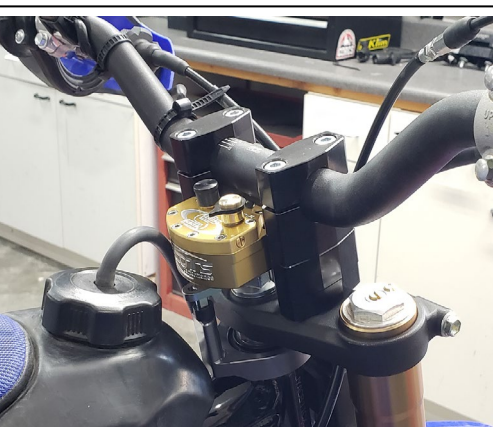
Install the Stabilizer so the tower pin is flush with the top of the link arm.
