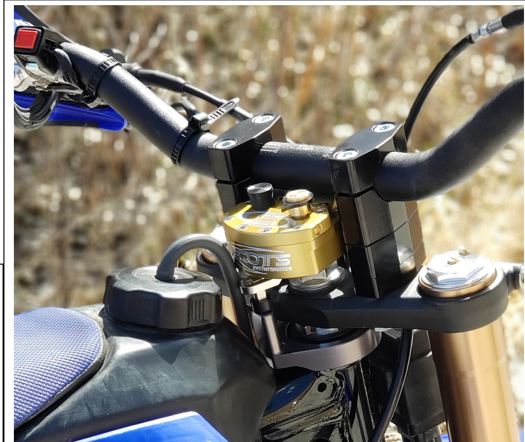
Tap the frame bracket down until the lip fits touches the head tube all the way around the top.
