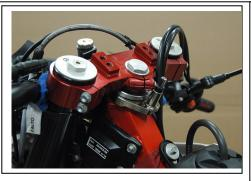
Install triple clamp & tension the main nut & fork pinch bolts to factory specs
