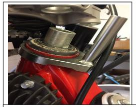
Keep the frame bracket low enough so when the shroud is on, no contact to the bracket.
