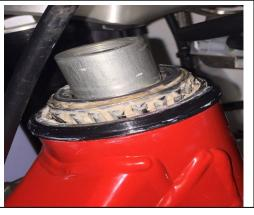
File any welds that keep the frame bracket from clamping tightly around head tube
