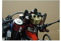
Install the upper half of the rubber sub mount to the base plate using the additional instructions provided to show that assembly in detail. Install the cable guide as per the photo below left.
