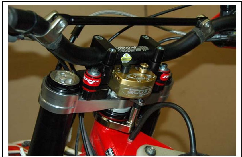
Using the additional instruction sheet, assemble the parts of the Rubber sub mount as shown
