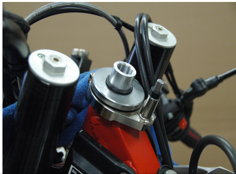
Install the Frame bracket first, then the new bearing shroud seal and finally the o-ring.
