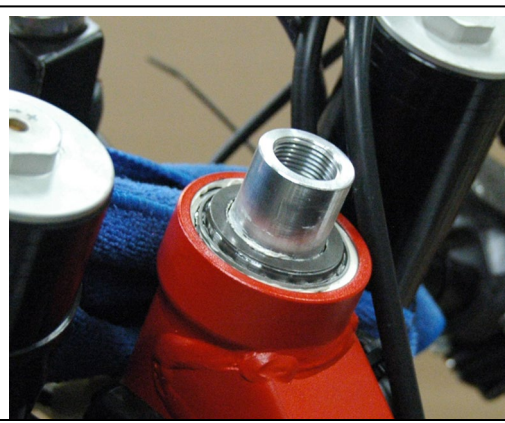
File any welds that keep the frame bracket from clamping tightly around head tube
