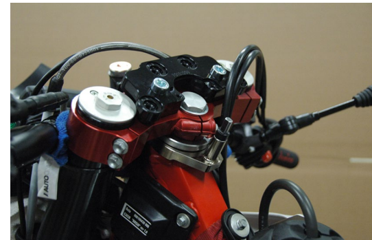
Install the base of the sub mount to the rear set of holes on 2 holes triple clamps and middle holes on 3 hole triple clamps
