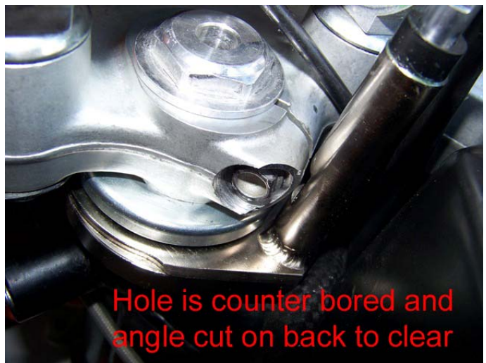
This shows where the bolt will approximately need to be after counter boring the pinch bolt hole deeper.
