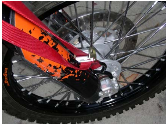
Hook a tie down around axle, up and over the frame
