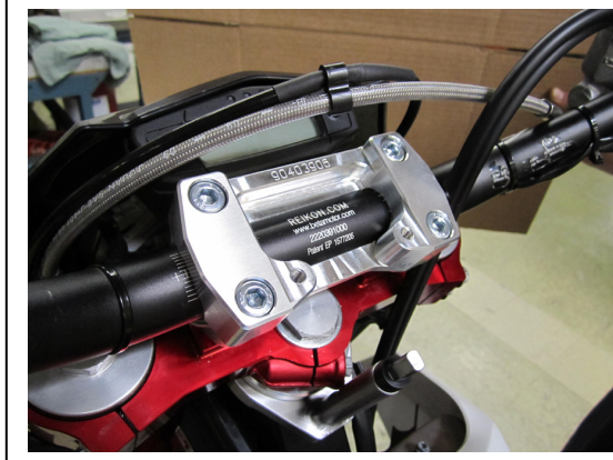
Be sure to have a minimum of 6mm from the top of the head tube to the top of the frame bracket
