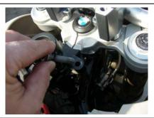
Stock key switch bolts are Torx remove and install frame bracket
