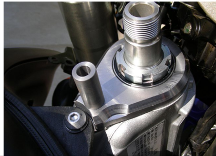
Slide the tab in under the tank first then the bracket over the stem, then tighten the castle nut .
