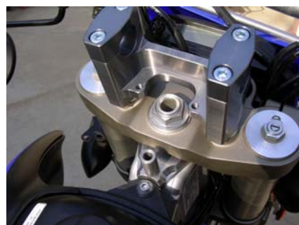
Sub mount installed on triple clamps
