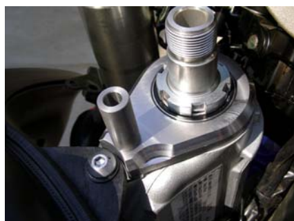
Slide the tab in under the tank first then the bracket over the stem.
