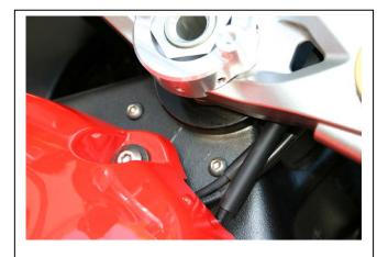
This photo shows the bike with the stabilizer kit removed and the holes plugged. We left them silver in the photo to show you how it looks, although the bolts could be black to blend with the frame.
