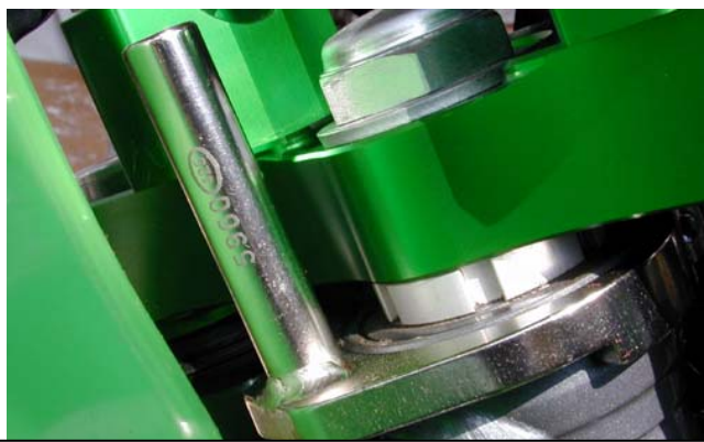
This shows the bracket flush with to top of the head tube
