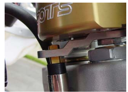
Correctly adjusted tower pin height
