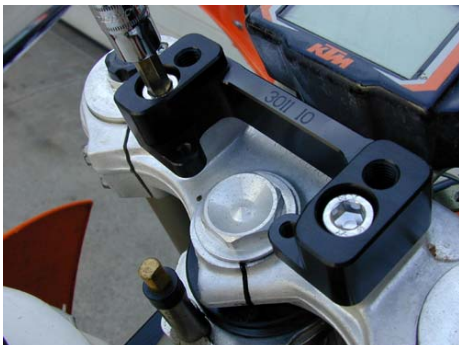
Note how the stabilizer bolt-holes are aligned over the steer tube center
