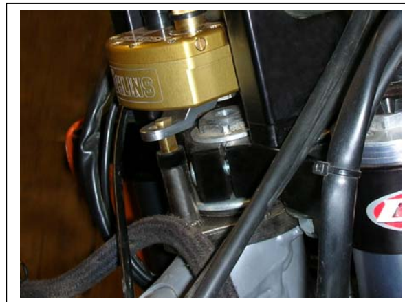
Key and cable guide on new triple clamp
