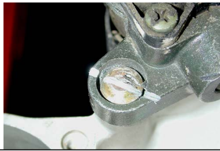
Cut a slot in the head for a screwdriver
