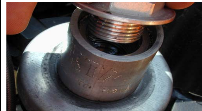
Spacer-tool to hold forks on while working with TC off.
