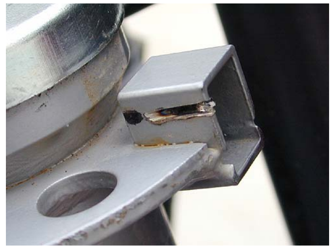
Use a hack saw or Dremel to cut the upper half off.
