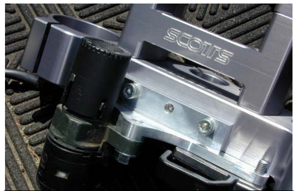
Key and cable guide on new triple clamp
