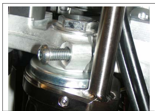
Select models may need the special low profile bolt for additional clearance.
