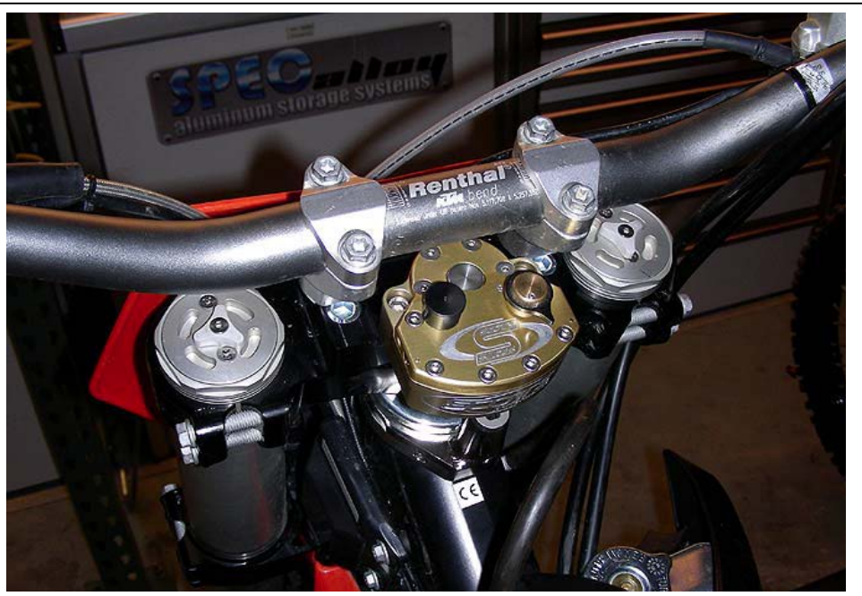
Bolt the SUB mount to the triple clamp Using the Allen Bolts provided
