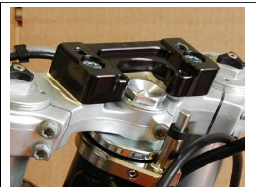
Bolt the SUB mount to the triple clamp Using the Allen Bolts provided
