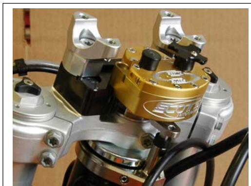
Bolt the stock barclamps to the SUB mount, using the Ktm Allen Bolts.
