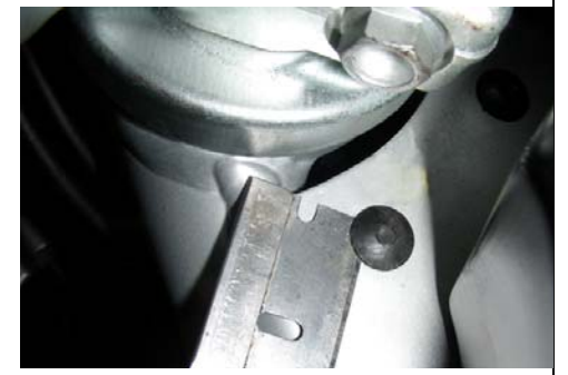
Remove plastic covers to expose bkt holes
