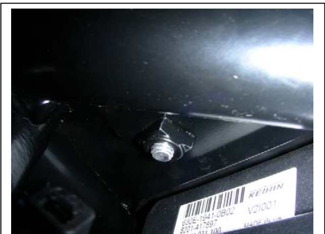
Nut located under the frame that tank bolt goes into. Our washer (at right) goes over it this nut after the bolt is tight. An additional nut is supplied for our washer.
