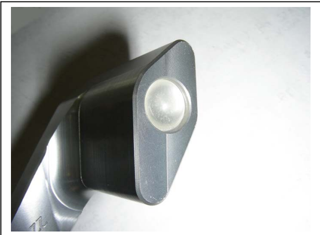
Install the rubber bumps onto the frame bracket feet
