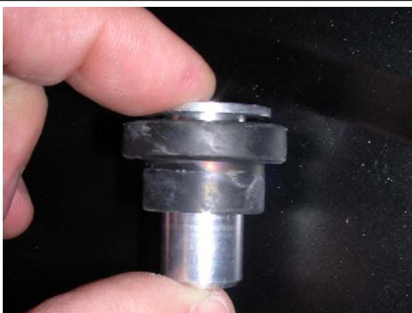
Install our new tank bushing through the stock rubber
