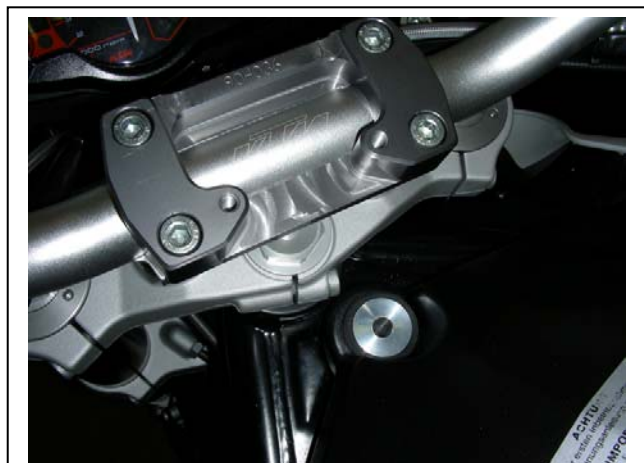
Barclamp and tank bushing installed
