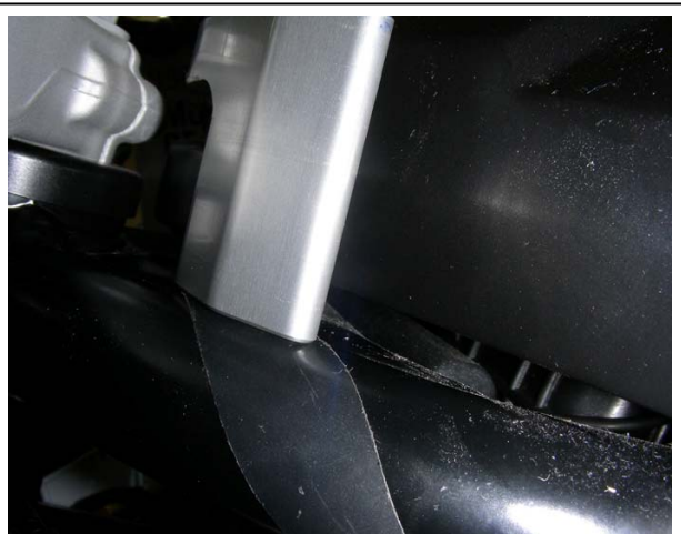
Be sure the bracket feet make contact with the frame
