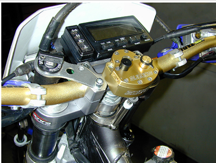
This shows the Reverse mounted position where no spacers are needed. DRZ-SM key switch mounts to upper left holes using 8x45mm Allens.
