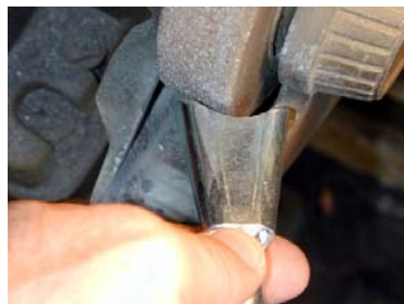
Shaping the base to match frame
