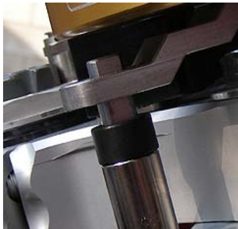
Tower Pin correct height after welding.
