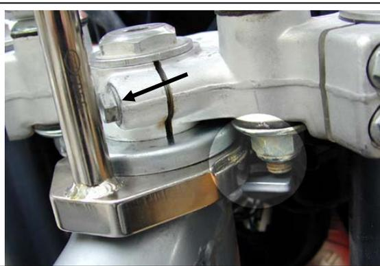
Where to file pinch the bolt area, if necessary.
